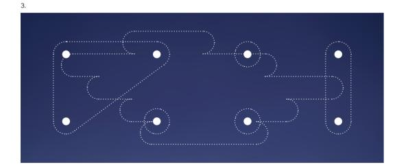
① Luminaire level: a single luminaire reacts (e.g., via sensors) to signals. ② Group level: the different luminaires communicate with each other – for example the sensor of one light can cause another to react. ③ Cloud level: not only can individual luminaires or groups be set locally, but they can also be controlled via software. > Video
